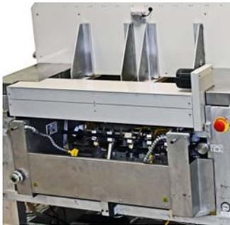
As with all the fully automatic functions of the AC-20X, the board feeder adjusts for size changes automatically to the precise specifications set by our program. This design provides very accurate registration of board and spine to cover sheet and eliminates errors.
