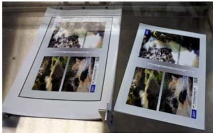
The cut size of each sheet can differ as the machine will register the cut locations by sensing the preprinted borders of each successive cover sheet and then cutting away the excess material.
