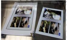
The cut size of each sheet can differ as the machine will register the cut locations by sensing the preprinted borders of each successive cover sheet and then cutting away the excess material.
