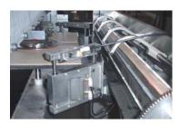
With delivery of cover components at exactly the time and in the right location for the operator, GP2 customers can produce more high quality covers per hour than ever before. Based on the well proven SC-2, the SC-3 features automated registration of the cover components and does not require the measurement of in-coming covers. The Corner Trimmer Option automatically trims the Corners from the cover material very accurately during the casemaking operation.
