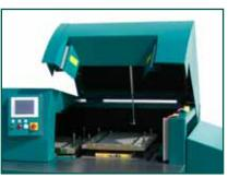
The state-of-the-art safety system of the machine (e. g. light grid) combines highest safety standards for the operator with perfect ease of operation as there are no disturbing coverings in the working area.
