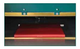
stop which is adjusted to the book size. The stop is released by push-button, aligned according to the book width and fixed at the correct position by the push-button. All further books is pushed against the stop only and is aligned properly.
