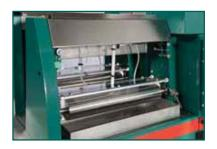
At the start of the operating cycle the blade is located in the upper position. A book block is opened in the centre, placed on the blade and pushed against the rear limit stop. The casing-in cycle is next triggered. The blade drives downwards between the gluing units.
