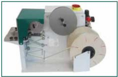
the width is the book block is measured and entered into the machine's control panel. The headband is guided automatically into the intake slot while being equipped with double-sided adhesive tape.
