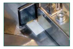
The book block is now placed into the intake slot against the stop and pressed down slightly, so that the headband sticks to head of the book block. By pressing the foot pedal, the headband is cut off at the pre-selected width. The block is now taken out. The next piece of headband is equipped with double-sided tape and forwarded into the slot. Now the next book block can be inserted and/or headband attached to the foot of the block just taken out.
